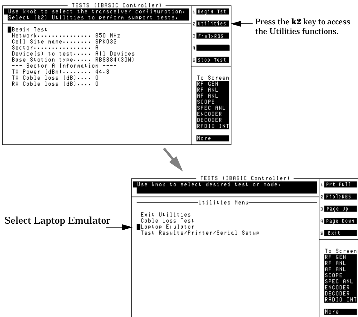
Figure 3-8 Accessing the Laptop Emulator from the Cell Site Information Menu
