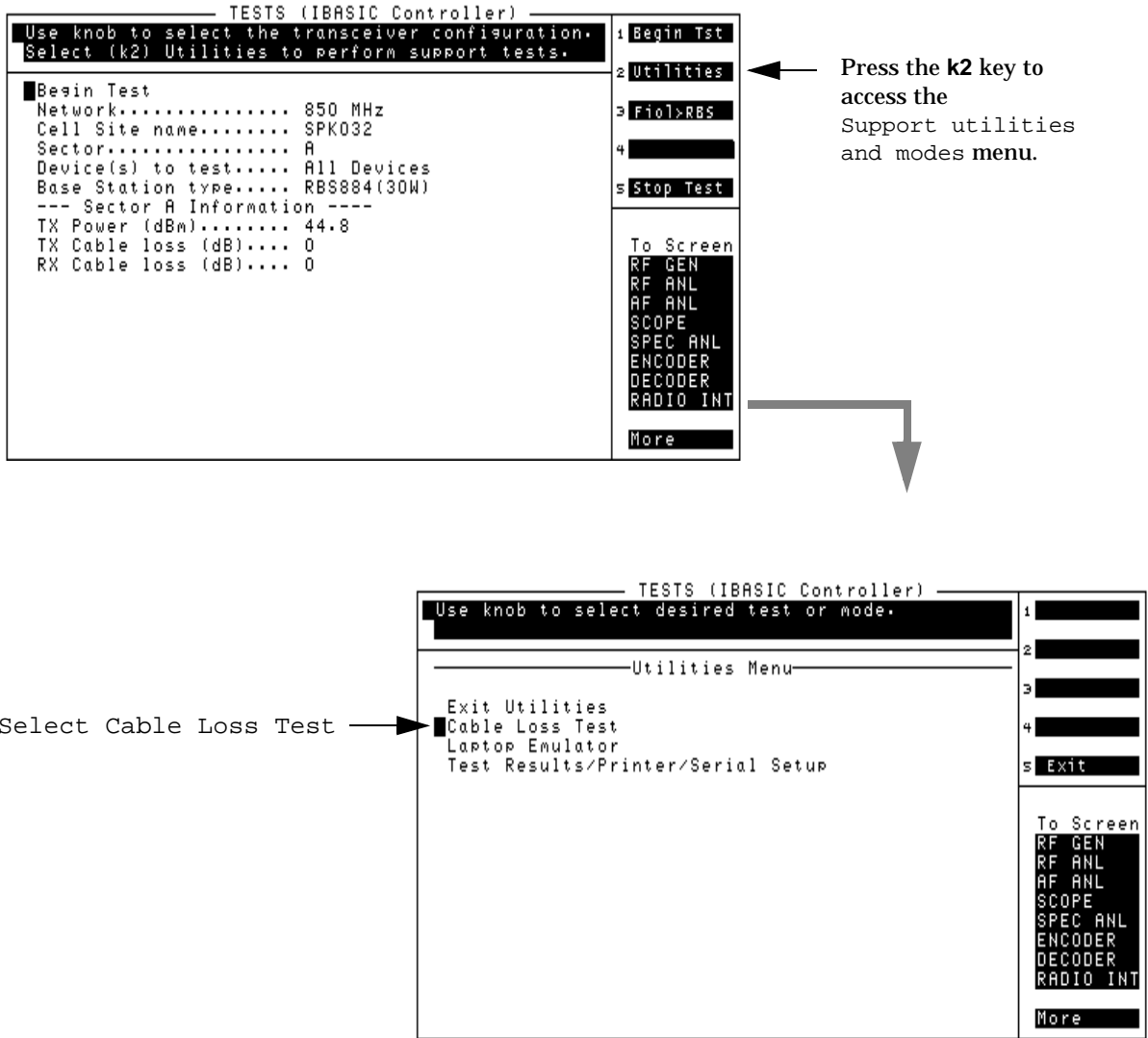
Figure 3-2 Accessing the Cable Loss Test
